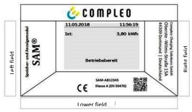
Figure 2: Type plate of the SAM (example)
